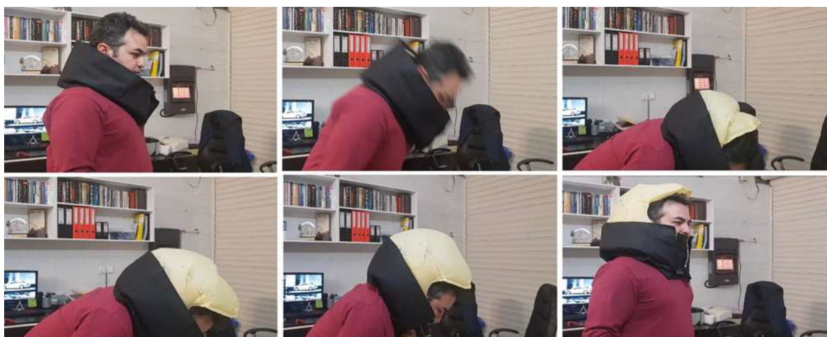
Fig 6 Procedures for testing an airbag helmet
