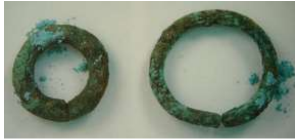
Fig 2 Corrosion products of bronze (Scott 2002: 186)
