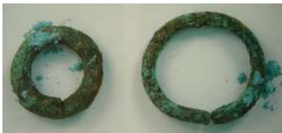
Fig 2 Corrosion products of bronze (Scott 2002: 186)
