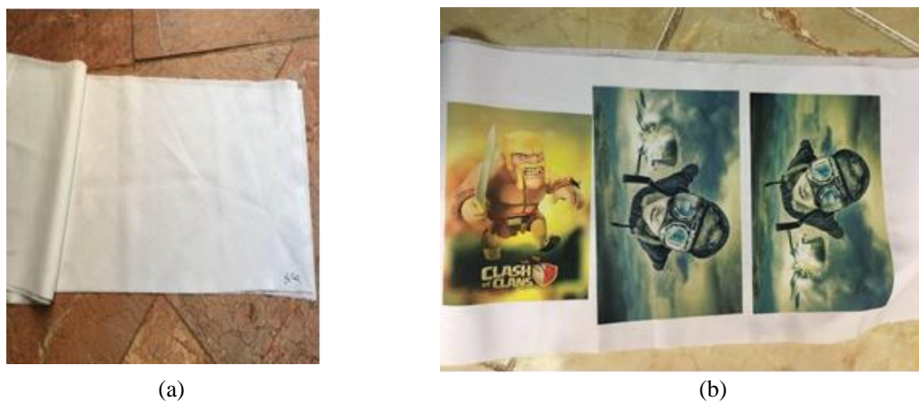
Fig 10 Polyester fabrics (a) control and (b) printed using sublimation printing
