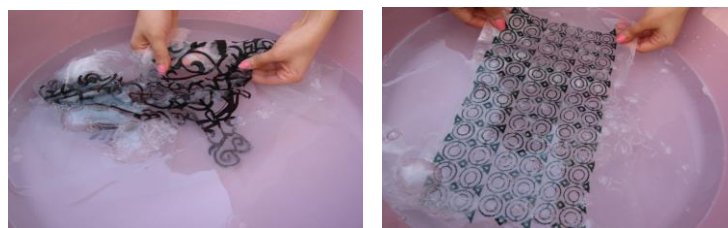
Fig 4 PVA fabric dissolving in water
